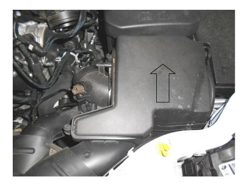
6. Using the cable tie provided secure the rubber intake scoop. Using a Knife or similar tool trim off any excess cable tie.
