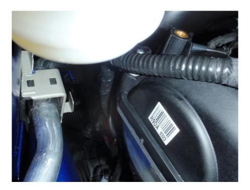
16. Place your Forge Induction pipe in position, connect the 19mm outlet to the open end of the silicone hose running from the cam cover, secure with a 25mm hose clamp. Bolt in place using the fixings provided.
