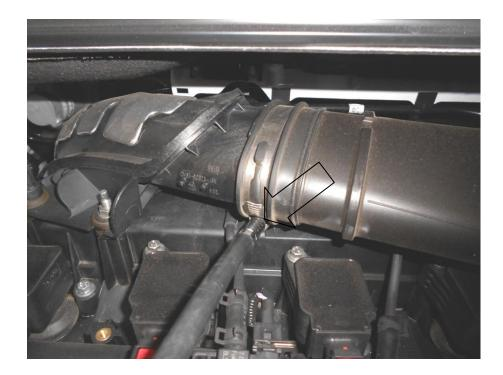
9. On top of the engine using a 10mm spanner undo the 1x nut.
