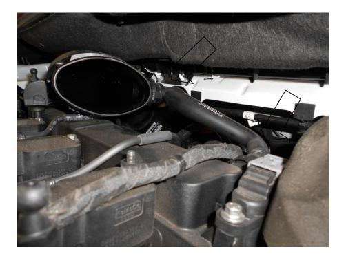
13. Remove the final part of the OEM induction pipework.
