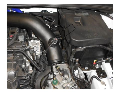
20. Secure the other end of the silicone reducer to the hard pipe with a suitable hose clamp.
