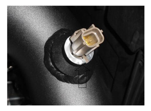
19. Reconnect the wiring to the sensor.
