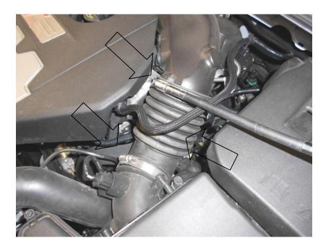
3. Carefully unclip the wiring to the sensor on the intake.
