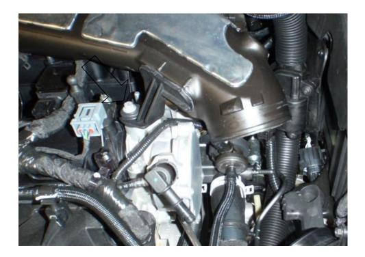
12. Unplug the standard engine breather pipe from the back of the cam cover and the side of the induction pipework.
