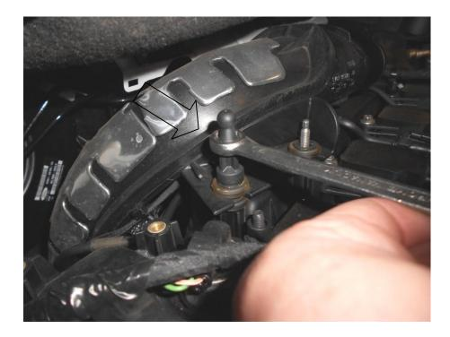
10. Using a 12mm spanner undo and remove the engine cover pin.
