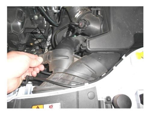
5. Pull the airbox up firmly to remove it.
